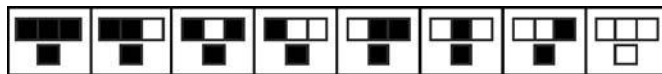
FIGURE 4-1 Graphical depiction of a one-dimensional cellular automaton state transformation function. A shaded square has state 1, an unshaded state 0.
